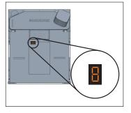
After a button is pushed, the scanner flashes the green LED a set number of times to indicate the error code. After one cycle of flashing has passed, another button push resets the scanner. The PRG describes the LED flash codes associated with an error found. If your scanner indicates any of these errors, note the code number, then contact Helpdesk for assistance.
